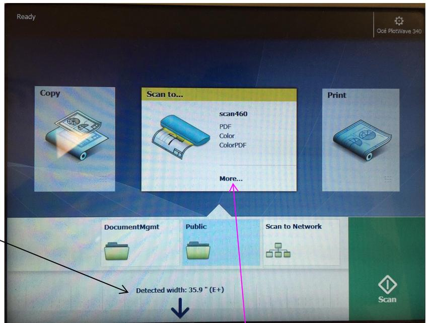
3a. Scanner will automatically "Detect Width"
