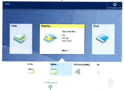
2. Select the 'Scan' tile on the user panel. The scan Smart Access is visible.
